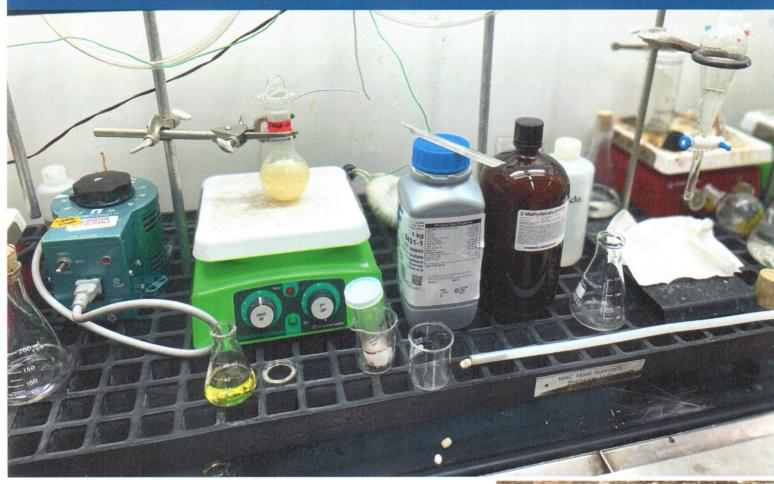
Multiple-Air-Channeling Hood Support (MHS) Safety Device **simultaneously elevates all equipment and chemicals** off the bench surface.
